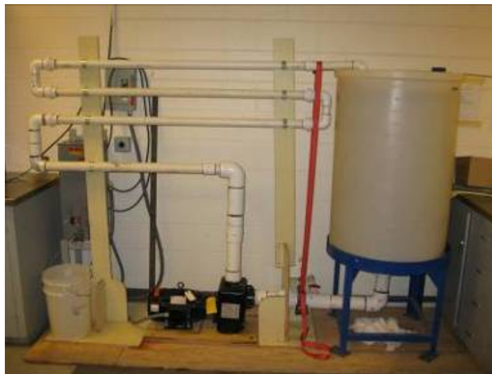
Figure 21.—High flow water test set up. Samples are placed inside 1.5-inch PVC pipe.
