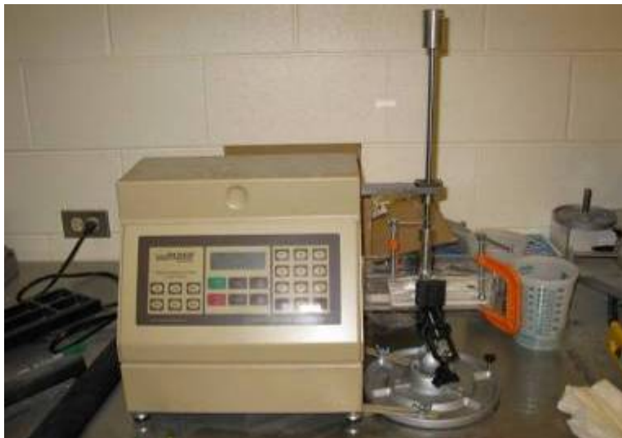
Figure 19.—Abrasion test setup.
