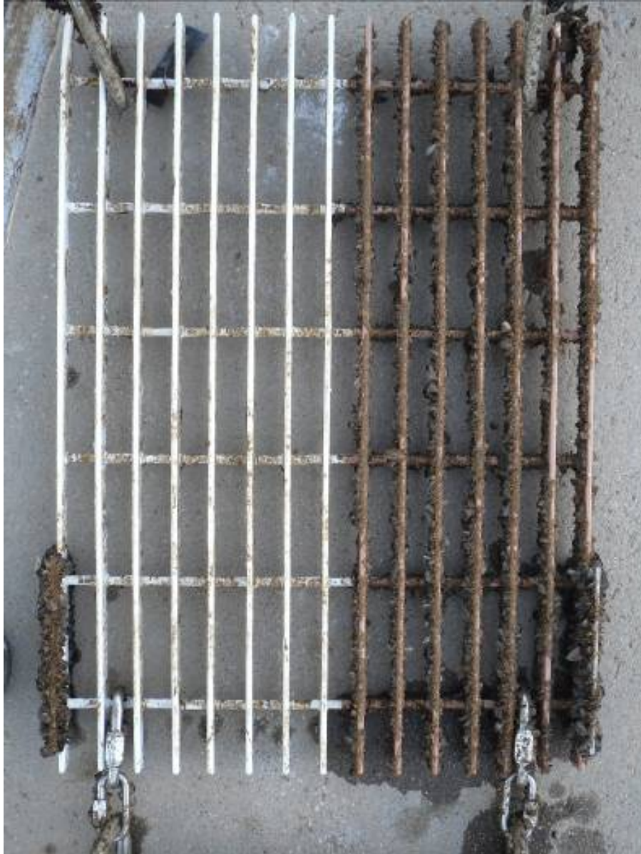
Figure 16.—Silicone FR #6 on the right and Silicone FR #7 on the left after 6 months in dynamic exposure (November 2010).
