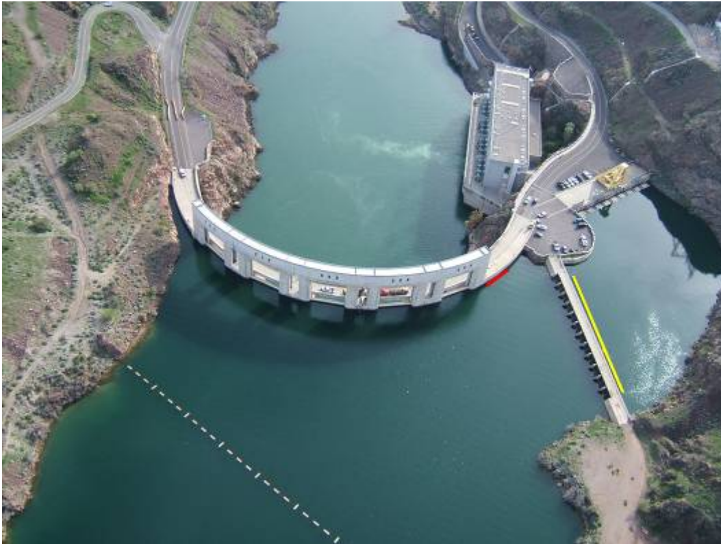
Figure 1.—Aerial photo of Parker Dam. The red line indicates the location the panels were placed, and the yellow line indicates where grates were placed.
