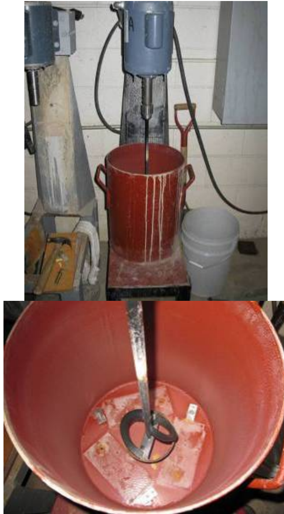
Figure 20.—Erosion test configuration.
