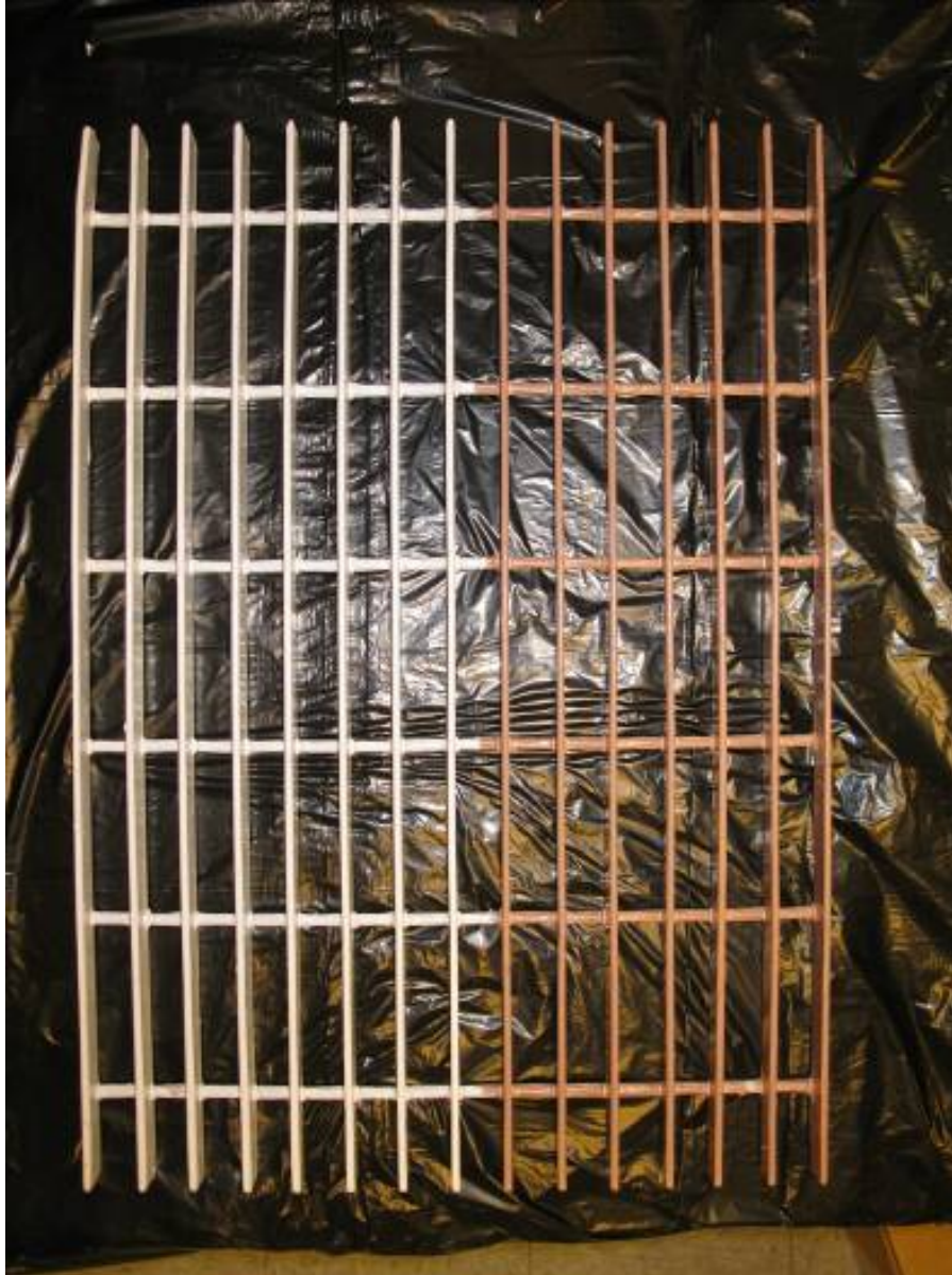
Figure 15.—Silicone FR #6 on the right and Silicone FR #7 on the left prior to exposure (May 2010).
