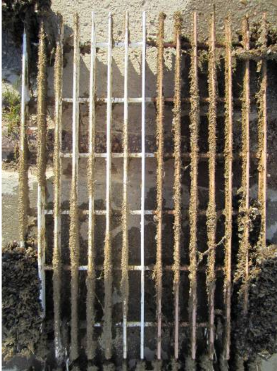
Figure 18.—Silicone FR #6 on the right and Silicone FR #7 on the left after 18 months in dynamic exposure (November 2011).
