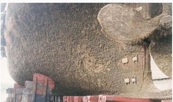
Hull fouling regulated under 3 discharge types
