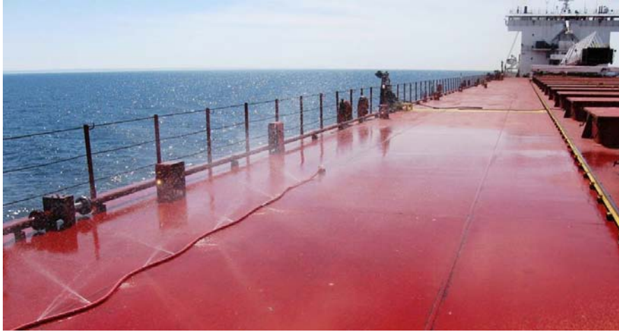
Photo 12 Testing the spray pattern of the perforated hose prior to in-tank test
