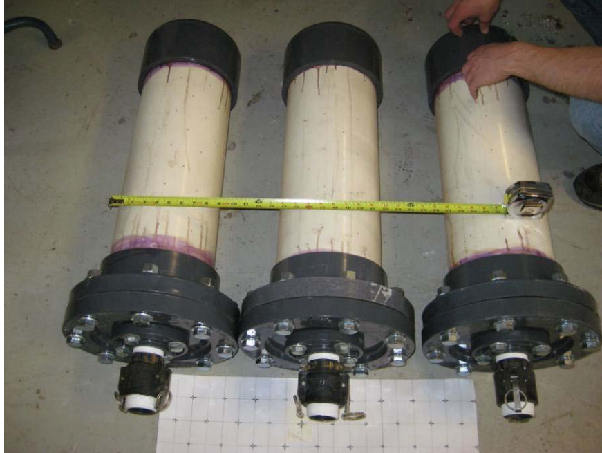
Photo 16 Point diffusers, 10" diameter pipes, 36" long, with ~100 holes each 1/8" diameter
