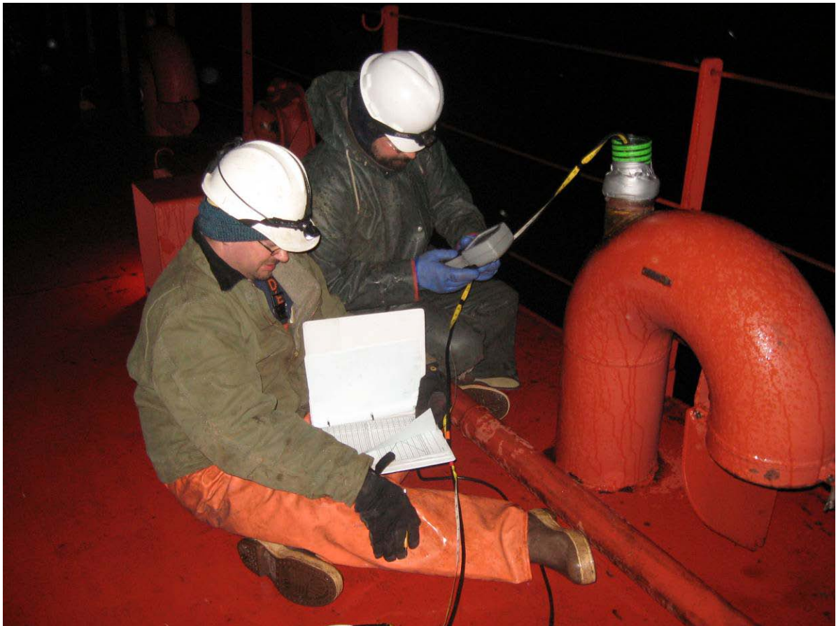
Photo 4 Tank Vertical Profiles - team members on vessel's main deck lowering sonde through fitting on tank vent and reading handheld data logger
