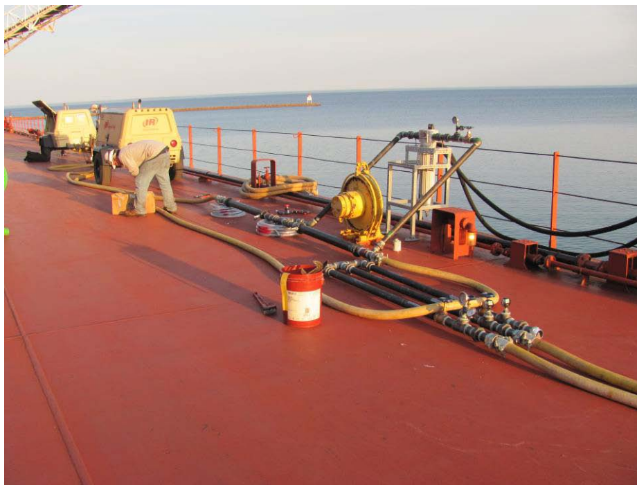
Photo 18 Air supply on deck for point and grid diffuser trials
