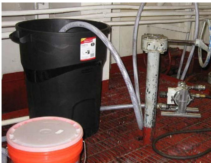
Photo 11 Phase II Trial Small Pump, Hoses, and Dosing Drum
