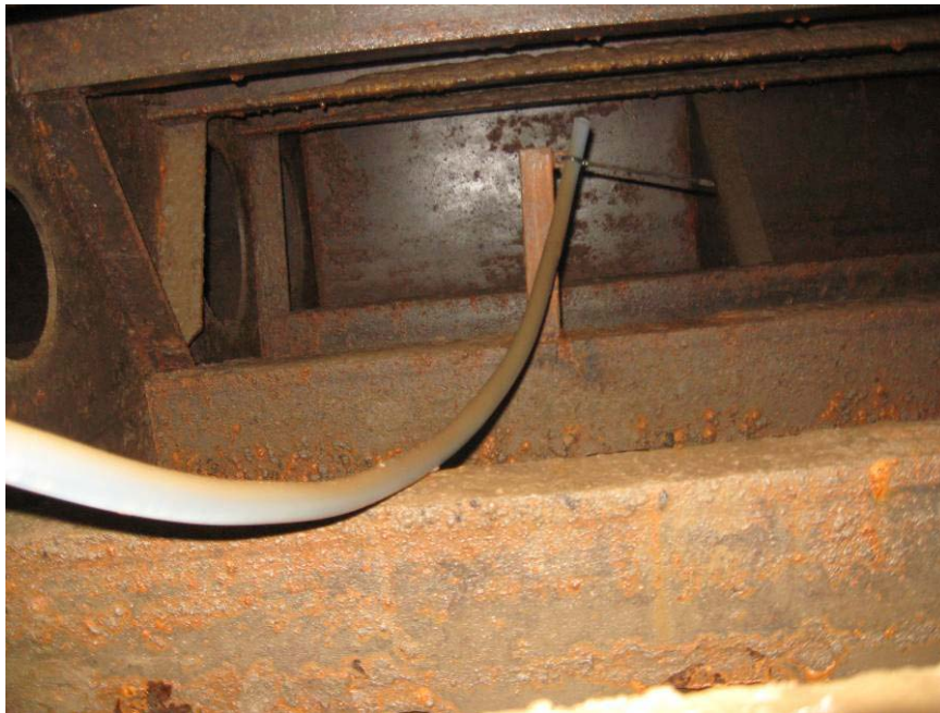
Photo 5 Discrete Sample Location—Open end of tubing secured at specific location within one of the six ballast tanks (one of sixty-two (62) locations)
