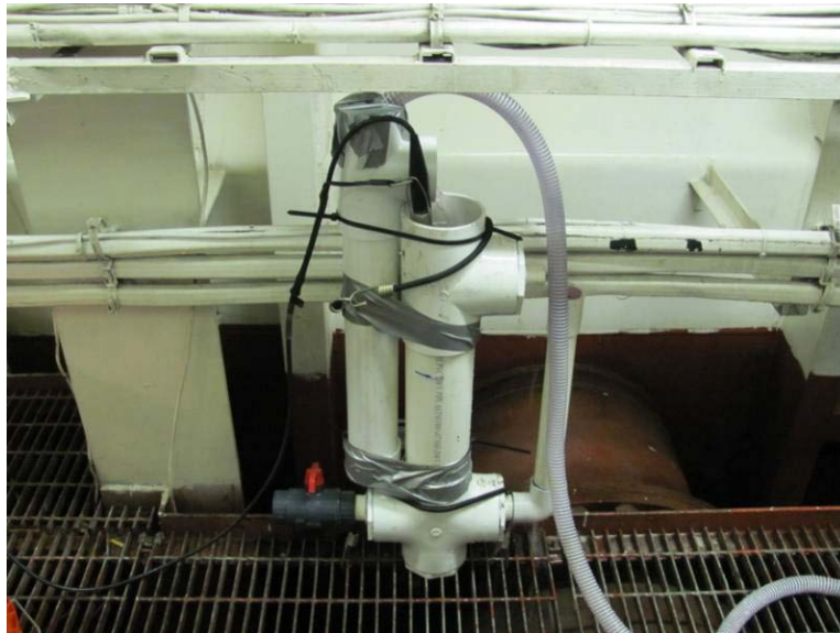
Photo 8 Discharge Monitoring Apparatus—Single hose supplies sample apparatus as ballast water is being pumped overboard (view from engine room)
