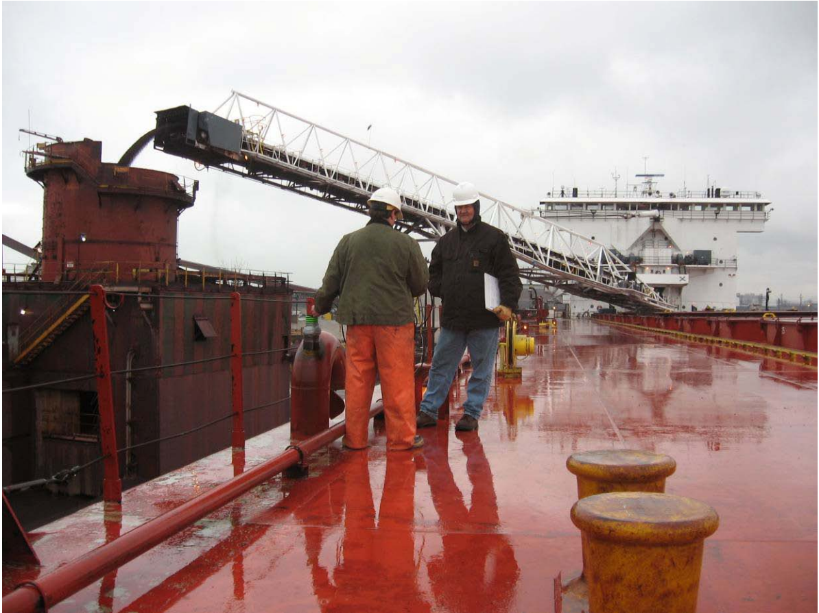
Photo 3 M/V Indiana Harbor, discharging cargo through loop conveyor system
