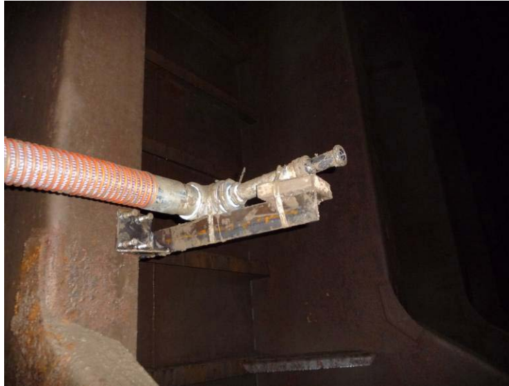
Photo 15 Nozzle mounted to vessel structure inside ballast tank
