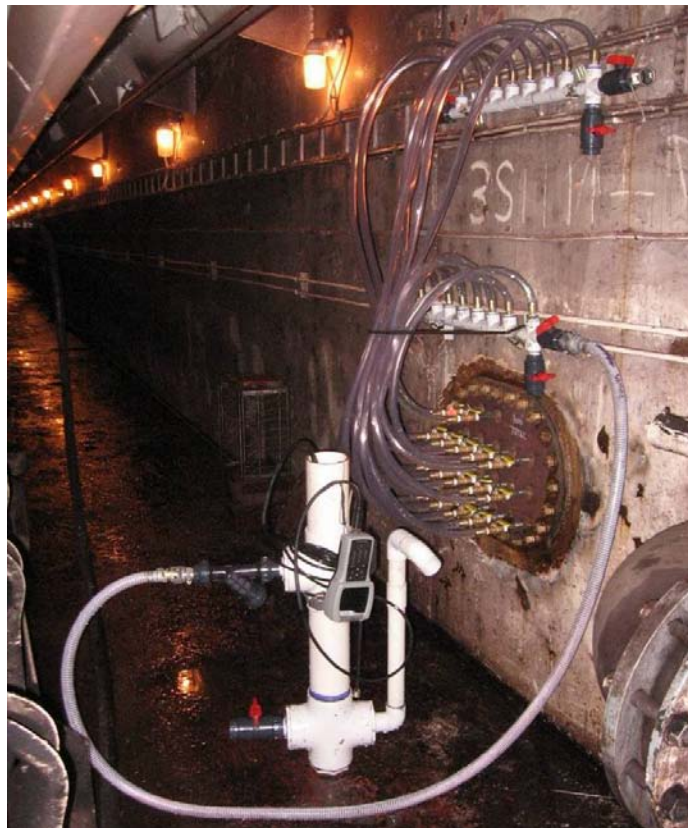
Photo 7 Discrete Sampling Apparatus and Arrangement—Valve and manifold arrangement allow direction of one discrete sample location to flow into the apparatus (view from conveyor tunnel, outside of ballast tank)
