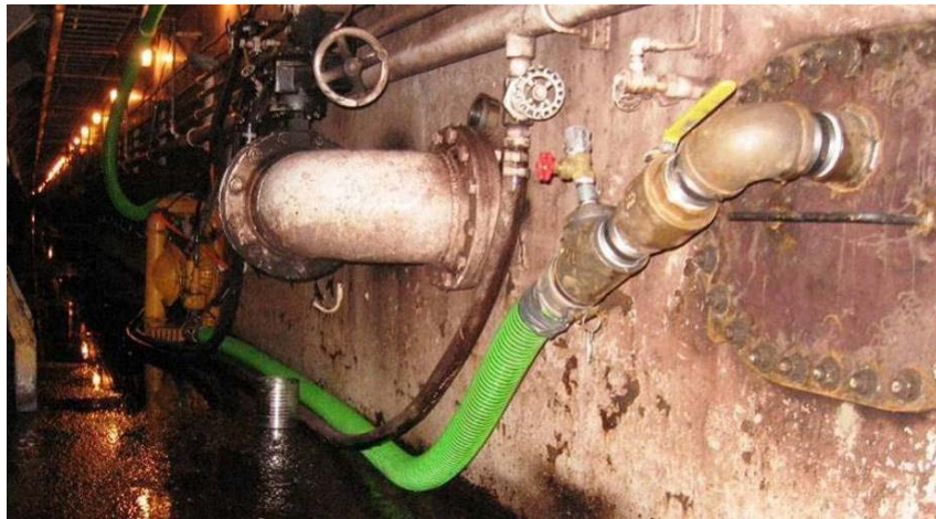
Photo 13 Internal transfer method, showing suction hose from ballast tank leading to diaphragm pump
