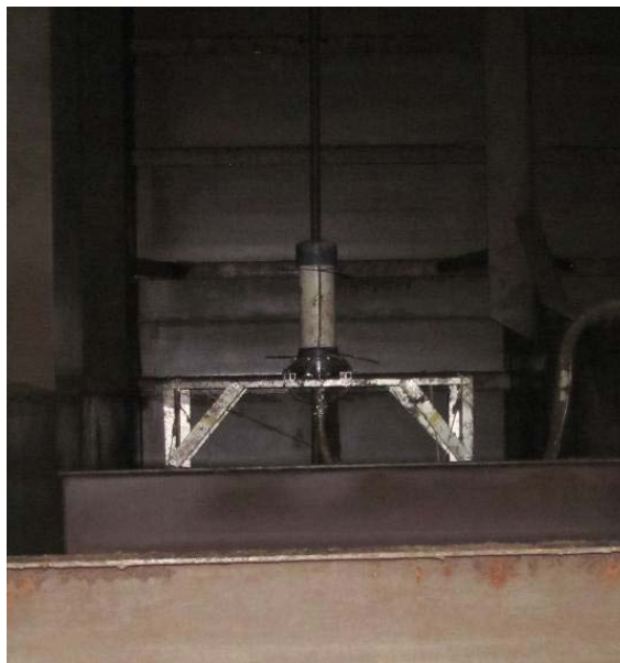
Figure 15 Point diffuser located in ballast tank
