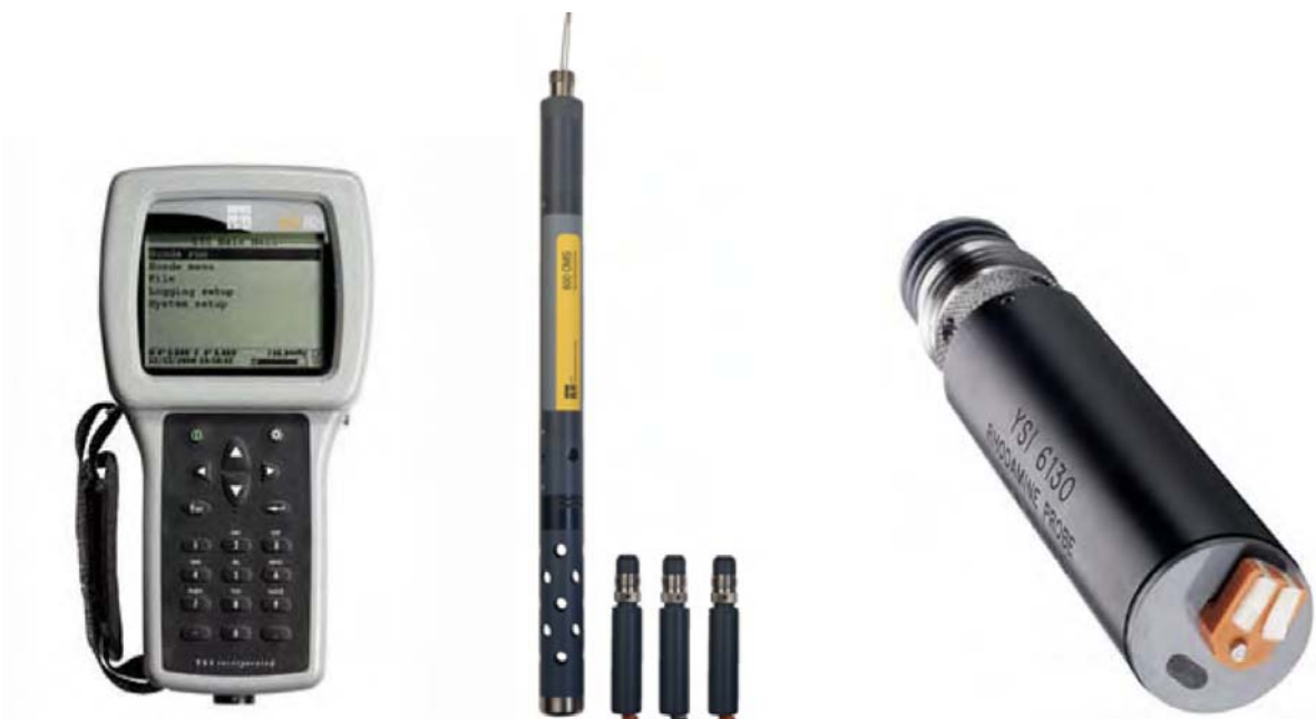
Photo 10 Sampling Instrumentation—YSI 650 Multiparameter Display System, YSI 600 Optical Monitoring System Sonde, and YSI 6130 Rhodamine Sensor
