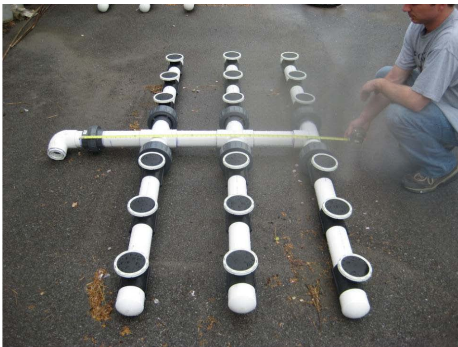
Photo 17 Grid diffuser, 18 course bubble puck diffusers
