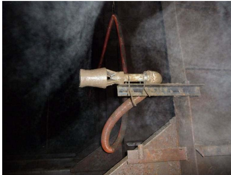
Photo 14 Eductor mounted to vessel structure in ballast tank
